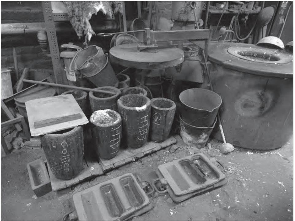
Collection of crucibles, each marked for their particular metal alloy ( Martin Snow )
