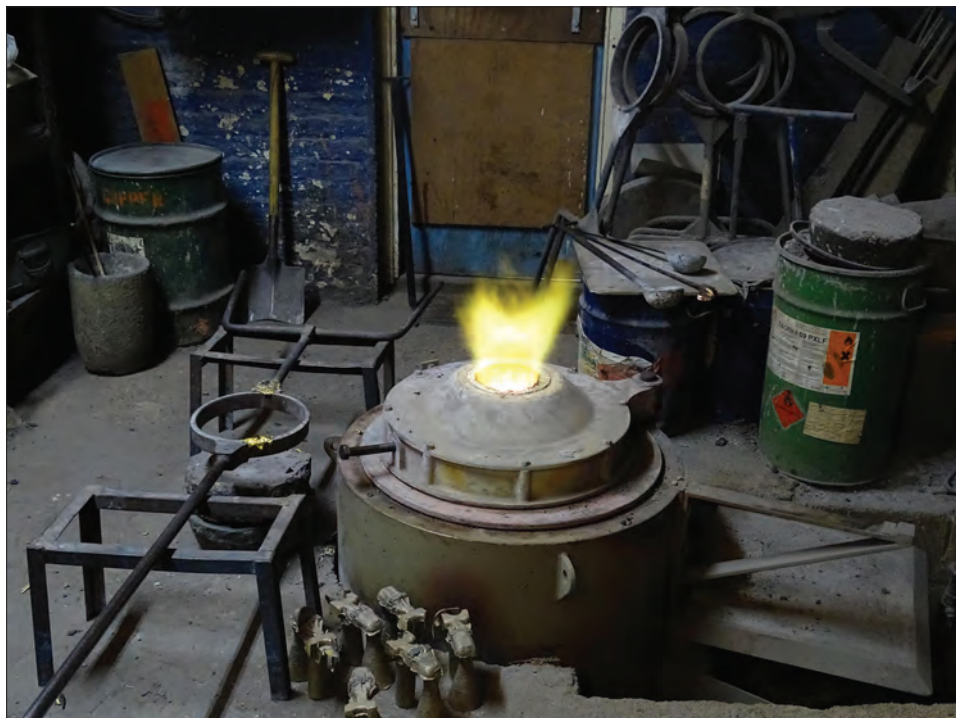
White Eagle Foundry visit. The gas fired furnace ( Martin Snow )
