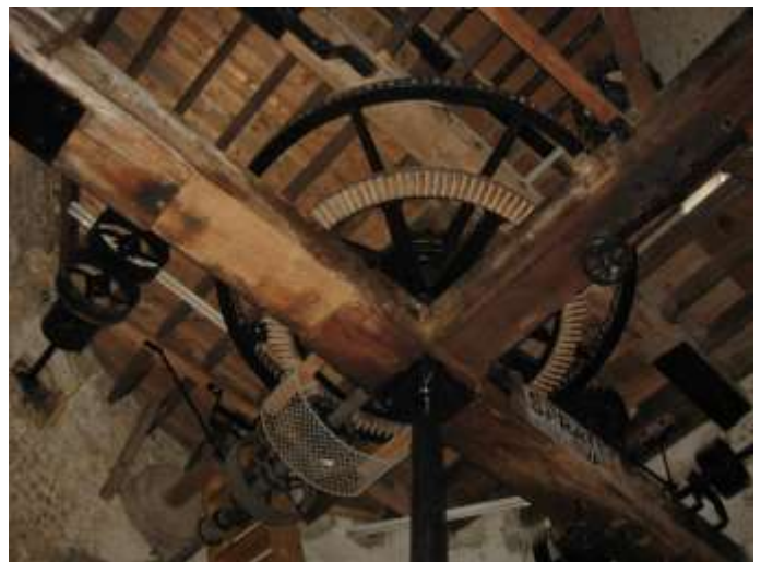
Fig. 5 Spout Floor prior to house conversion - showing the Great Spur Wheel, Stone Nuts and other surviving machinery, October 2010
