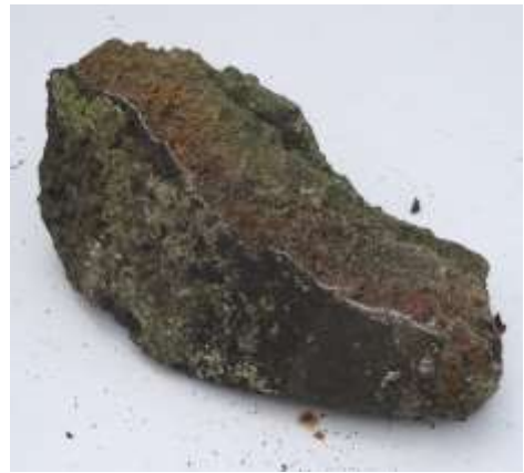
Fig 11. A piece of retort lining, once part of the gasworks wall which somehow found its way into the author's garden. The curvature can clearly be seen. (Author)
