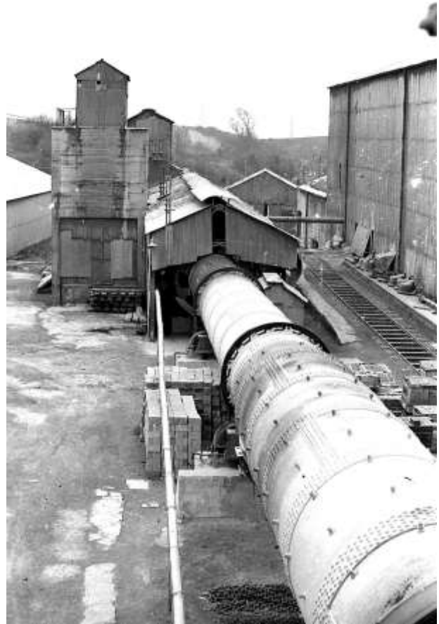
Fig. 4 Kiln showing tyres, clinker store to right, coal mill far structure in centre
