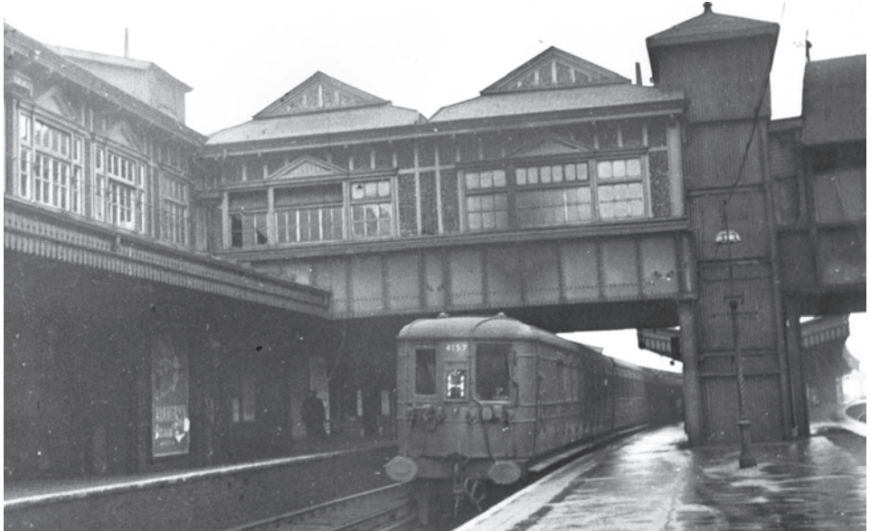
Forty years on and sixty years ago. A former LSWR suburban electric unit, now formed as 4 SUB no. 4157, arrives at Clapham Junction's platform 10 on a gloomy day in January 1953, bound for Waterloo. At this time the LSWR letter headcodes were still in use; in this case 'H' denoting the Hampton Court service. Headcodes of all varieties are now just a memory.
