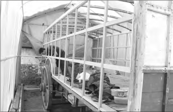
Fig. 11 Adrian Vaughan working on the framework of the van. The original woodwork was retained where possible.
