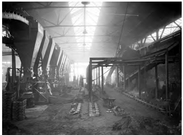
Fig. 8 The Mechanised Foundry with high pressure moulding machine to the left with sand hoppers above. ( Edward Reeves, Lewes )
