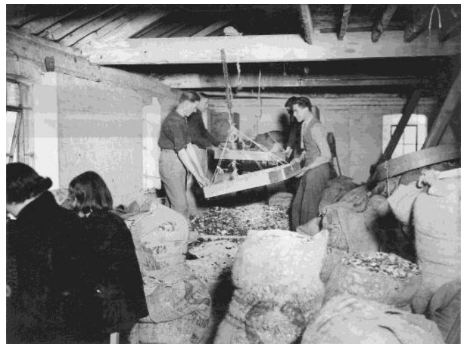
Fig. 5. Giovanni Donati on the right, manager of the colouring and polishing department on the top floor of the warehouse adjacent to the corn mill, assisting his staff to sieve and sort a consignment of semi-finished buttons imported from the Continent.
