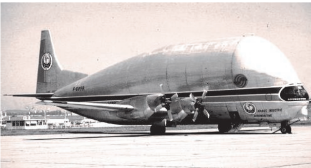
Fig. 8 The Super Guppy Transport Plane, used to transport Airbus components between European factories
